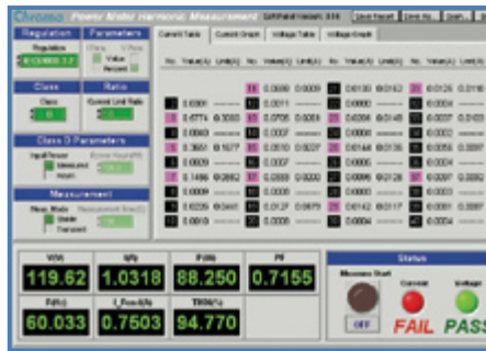
IEC 61000-3-2 Current Harmonic Test
